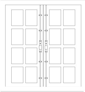
Joseph Giles Cremone Bolts are fitted with a unique non-handed rack & pinion gearbox mechanism which provides a 90 degree movement of the knob and a 13mm throw of the rods into the top and bottom of the door frame.
