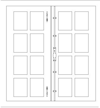
Joseph Giles Cremone Bolts are fitted with a unique non-handed rack & pinion gearbox mechanism which provides a 90 degree movement of the knob and a 13mm throw of the rods into the top and bottom of the door frame.
